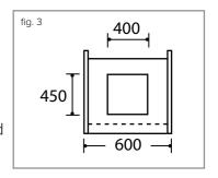
Ensure that air can flow freely around the housing area. If the oven is being installed into a fully enclosed built-under oven housing unit it may be necessary to cut a small slot in the top of the plinth fitted under the unit. Cut a section 400mm wide and a minimum of 15mm high to allow air to pass under the unit. Alternatively cut a section 400 x450mm in the base of the carcass as indicated.
