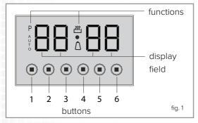
To confirm a selection when programming the clock/timer, once the display shows the preferred selection, simply do not touch any further keys for approximately five seconds. The oven will automatically confirm the selection.
