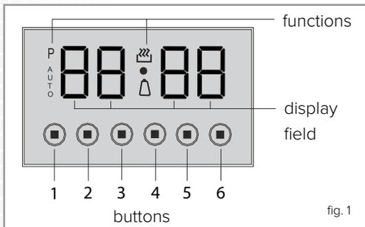
To confirm a selection when programming the clock/timer, once the display shows the preferred selection, simply do not touch any further keys for approximately five seconds. The oven will automatically confirm the selection.
