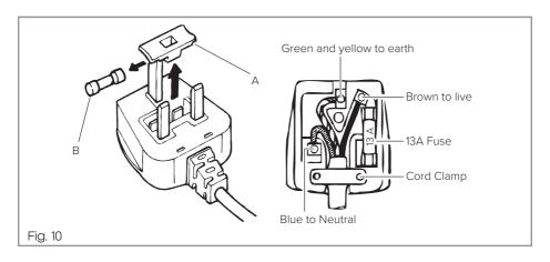
The mains lead of this appliance has been fitted with a BS 1363A 13Amp fused plug. To change a fuse in this type of plug, follow the steps below:
