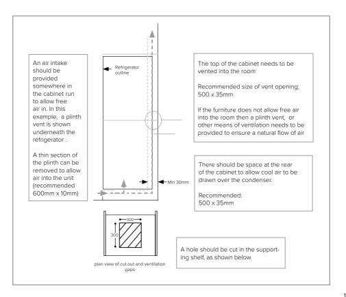
The open channel at the rear is clearly shown. For the correct operation of the appliance it is important that the top of the housing unit is not blocked off. A channel depth of 40-50mm is normal with most units.
