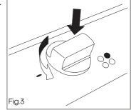
hold down the control knob to begin the ignition process (a clicking sound will be heard). Hold down the control knob for a few seconds after ignition to allow the safety device to detect that the burner is lit.
