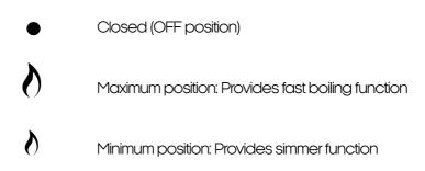
The hob can be set to the desired position by turning the control knob through the adjustment range in an anti-clockwise direction.
